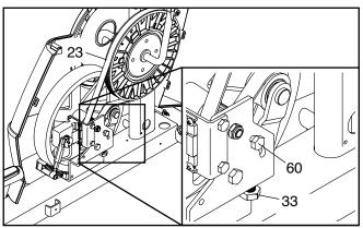
When the Drive Belt (23) is tight, tighten the M6 x 20mm Hex Screw (60).
